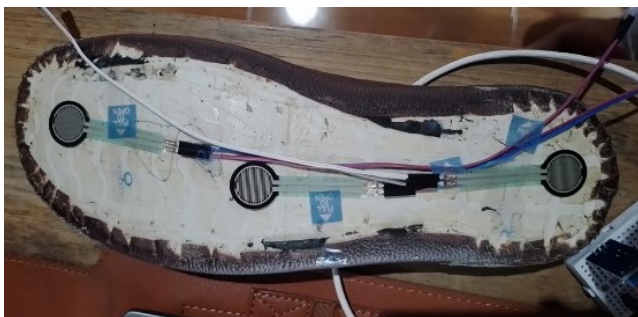
Fig. 4. Installation of Pressure Sensors
